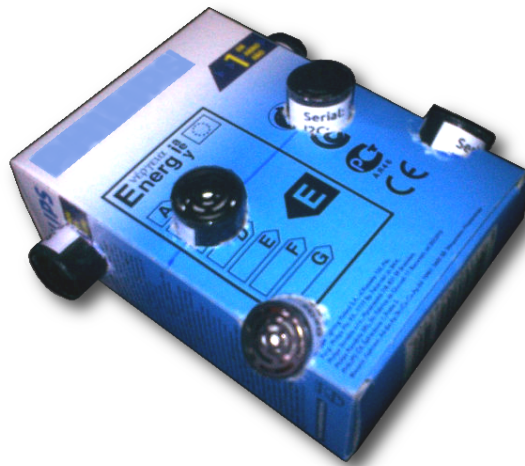
Figure 4.2.: Ultrasonic sensor array, consisting of six sensors
